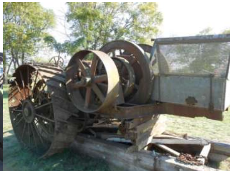
This rare Fairbanks Morse tractor came out of Angleton. It had been used as a stationary engine.
