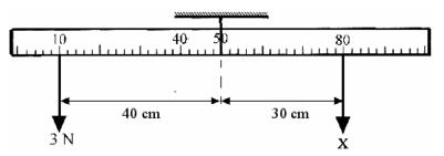
A uniform metre stick, suspended at its mid-point is balanced as shown. Calculate  $\emph{force}$  X.
