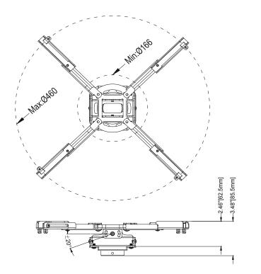
Heavy duty all steel construction in a very low profile package. Multiple (12) adjustment points for extra grip with heavier or off-center of gravity projectors. Comes completely pre-assembled for a quick installation and features a quick release for bulb replacement.
