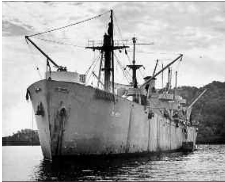
USS Serpens at anchor somewhere in the Pacific islands with derricks extended to take on cargo. (U.S. Navy)
