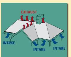
Research has shown that the best way to ventilate an attic is with a *balanced system* of intake vents low at the roof's edge or in the soffit/eaves along with exhaust vents high on the roof at or near the ridge. This allows cool, dry intake air at the roof's edge to flush out any warm, moist air through the exhaust vents
