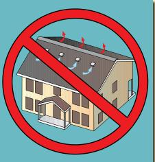
One of the most potentially troublesome attic ventilation mistakes is having two different types of exhaust vents on your house—for example, mixing a ridge vent with a powered fan, a roof louver, a gable louver or a wind turbine. Technically, this mistake is called short-circuiting the attic ventilation system. (See illustration on the left.)
