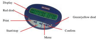
The diodes show the status of the Heliprobe<sup>™</sup> Analyzer:
