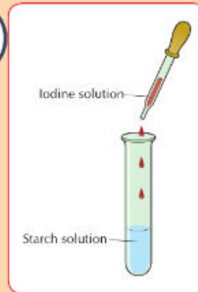
Fig. 4.7 Testing for starch.
