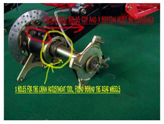
The brass colored tool as pictured below is for the chain adjustment. Too adjust your chain, simply jack up your Buggy off of the floor, and please keep in mind that with the rear wheels up, the Buggy will roll, so please block the front wheels. Now loosen the 6 allen head bolts from the rear of the swing arm.
