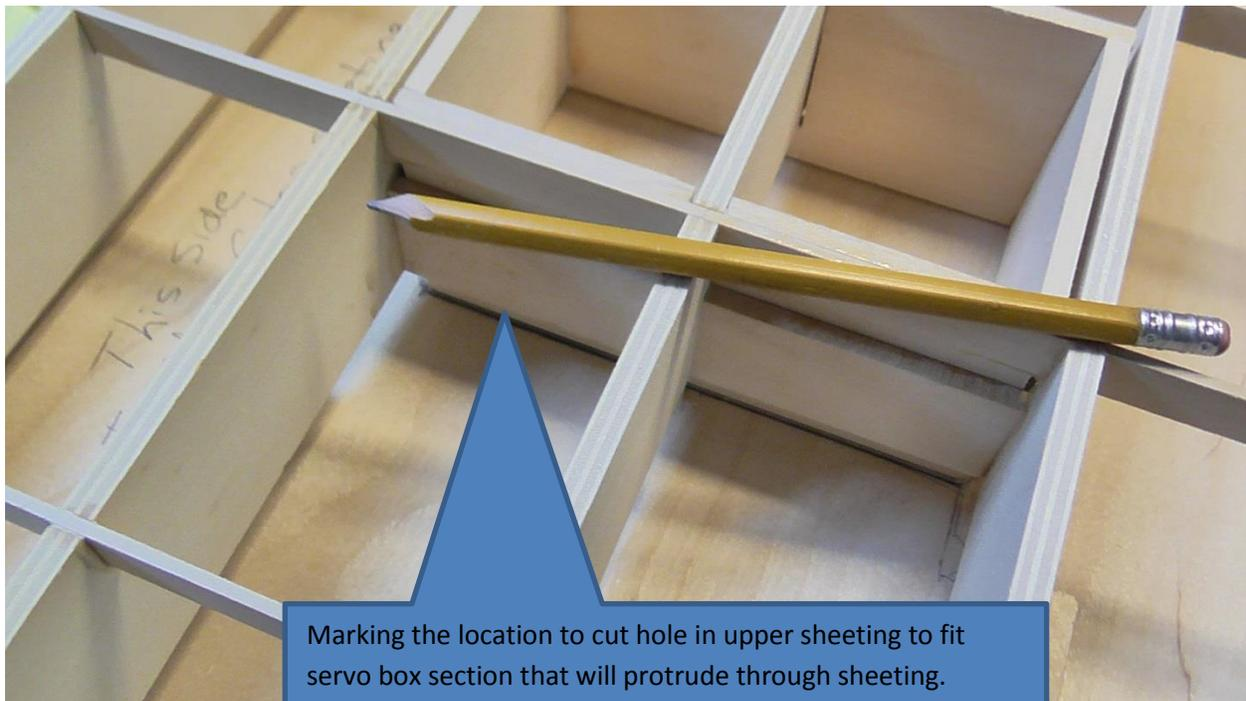
Marking the location to cut hole in upper sheeting to fit servo box section that will protrude through sheeting.
