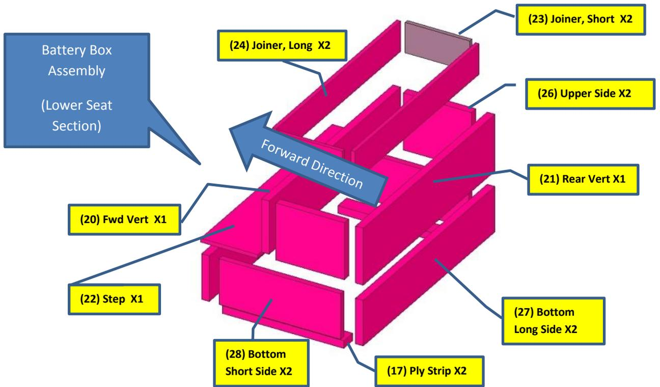
14. Assemble the Battery Box / Seat:
