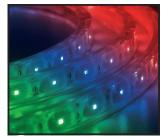
The same Cove Light we also offer in 11\*18mm RGB, so that you can create any imaginable color. The maximum length in one line for this model is 20 meter, the cutting distance is also 20cm and this rope contains 36 LED p/meter as well. Power consumption is 6 Watt p/meter. Cove Light SMD works on 24V.
