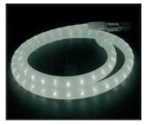
Cove Light Round has a modest light intensity for use in luxury yachts and living rooms. It is based on rope light (13mm round rope) but with a higher quantity of LED (60 LED p/meter compare to 36 LED p/meter for regular rope light) and has a diffuse coating over his surface, to avoid shading.
