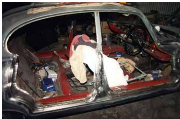
The interior was completely stripped and all the paintwork was taken back to bare metal.
