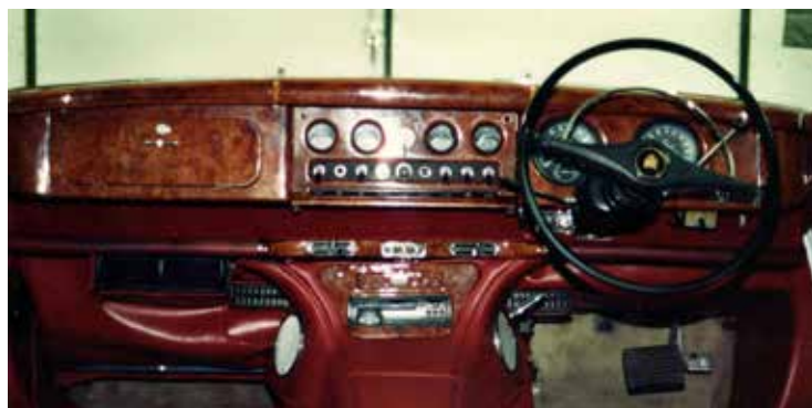
All woodwork was removed, sanded and clear coats progressively added over a 12 month period.
