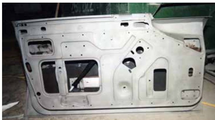
All panels were sand blasted, repaired and primed.
