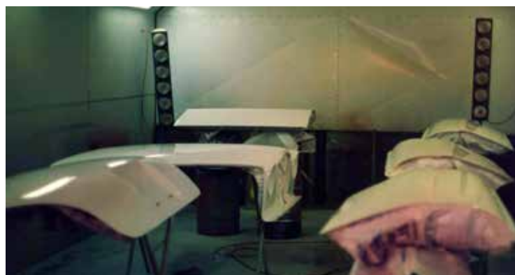
After the front/rear suspension were rebuilt the body, shell, engine bay and panels were all repainted.
