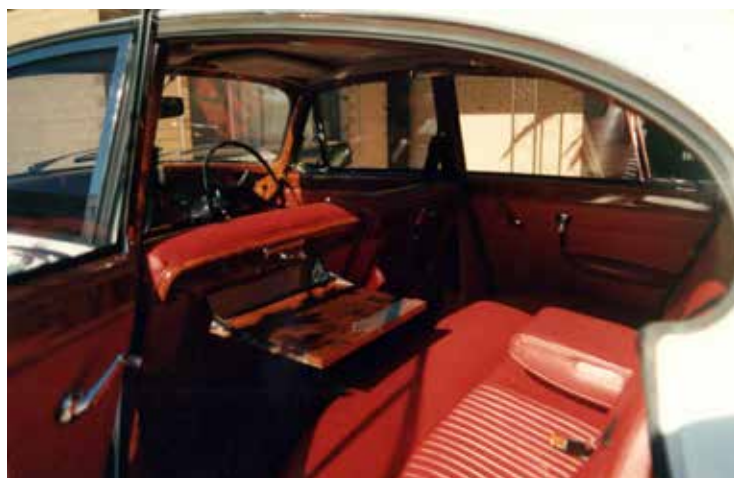
All the interior was re-trimmed and a second level was installed in the boot compartment and carpeted.
