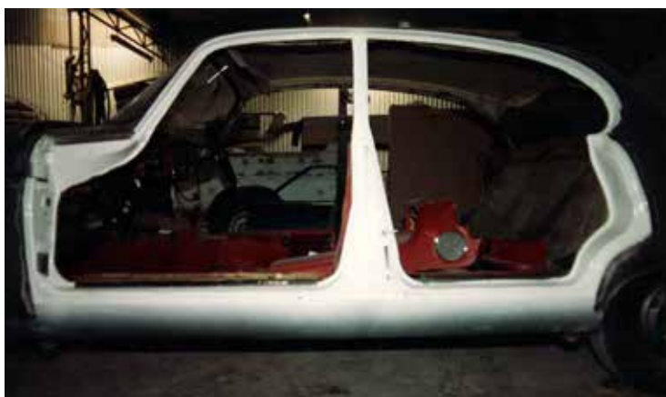
All panels were sand blasted, repaired and primed.
