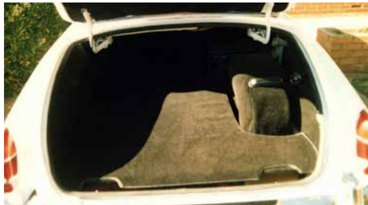
All the interior was re-trimmed and a second level was installed in the boot compartment and carpeted.
