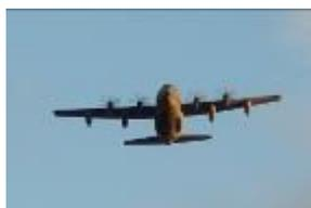
campsite, but possibly trying out various flightpaths into RAF Mildenhall, some eight miles away. It is powered by four Rolls-Royce AE 2100 D3 turboprops (for those passionate to know) and performs with some grace despite its unladen weight of 34,000 kilograms. As we found out, it can cruise at 300 feet without really much noise, considering.
