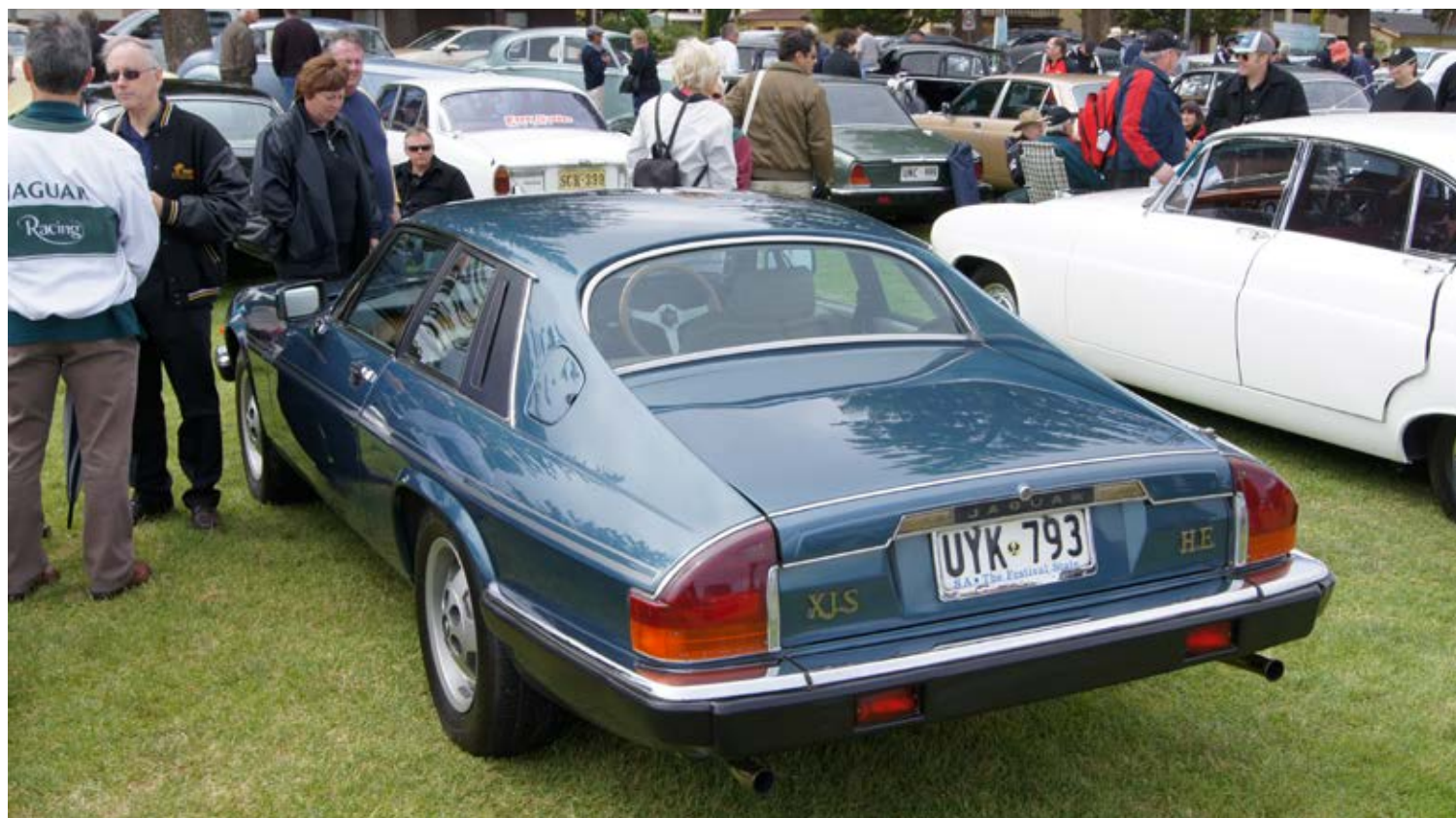
Ivan and Janine Cooke's 1984 XJ-S HE. Obvious changes over a pre-HE model include chrome inserts on the upper part of the bumpers, five-spoke (starfish) alloy wheels and the HE badge on the boot. (Photograph taken SA Jag Day 2010).
