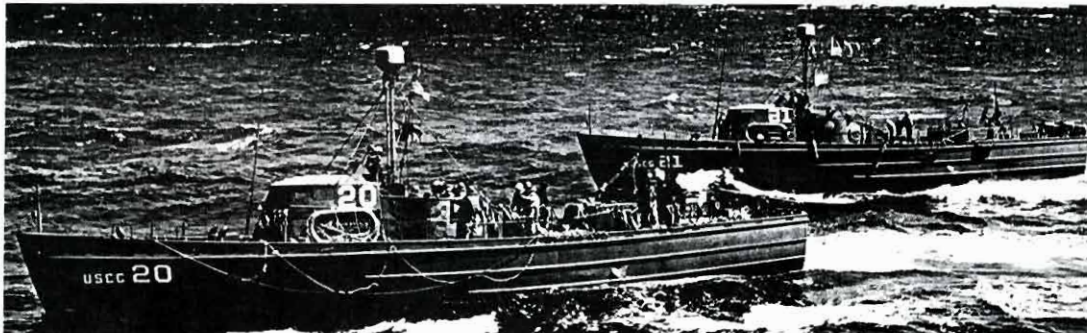
CGs 83401 and 83402, wearing their invasion markings, served as rescue boats during the Normandy landings. The sloping bridge face and the rounded bridge roof were common features of the earlier versions of 83-footers.
