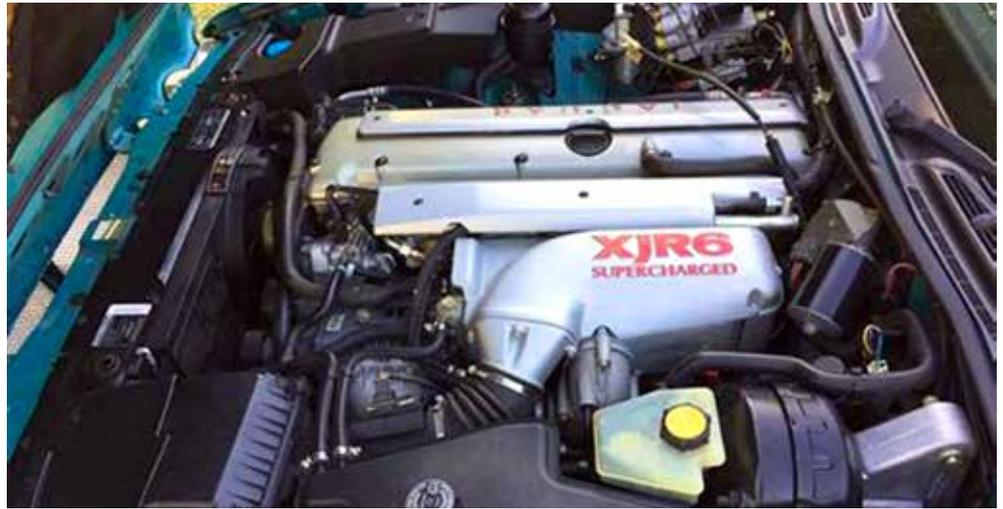
*1995 XJR supercharged AJ16 engine producing 326 hp (243 kW; 331 PS) and 378 lb-ft (512 N-m) with the use of an Eaton M90 supercharger and an air-water intercooler.*
