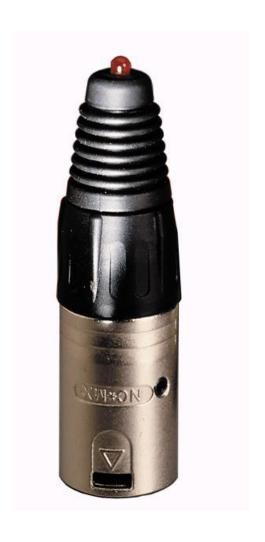
**PRODUCT DESCRIPTION:** A microphone input tester consisting of tone generator and phantom power detector built into a standard 3 pin XLR male connector. When inserted into a microphone input connector, the LED indicator will light showing that there is a phantom power voltage present. If a voltage is present, a 1kHz tone will be sent into the microphone input.
