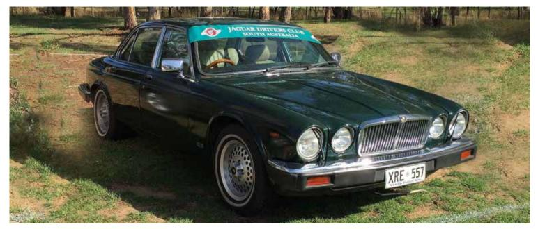
1985 Series 3 XJ6. The most obvious changes were the injection-moulded black bumpers with integrated indicator lights, flush door handles for increased safety and a revised roofline with narrower door frames and increased glass area.
