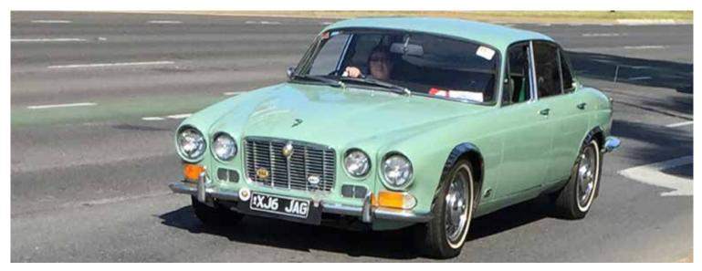
1971 Series 1 XJ6 featuring the deeper grille, slender bumpers and chrome overriders. Production changes in 1970 included modifications to the front wheel arch flanges to provide better tyre clearance.
