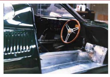
The inside of the XJ13 was pure racing car with bare aluminium, no insulation and aluminium radiator pipes running above the passenger floor.
