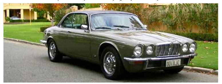
1978 Series 2 XJC. To comply with US safety regulations, a higher front bumper and smaller grille was fitted. The overriders became 'underriders' flanking a prominent rectangular air intake with indicator lights under the bumper.
