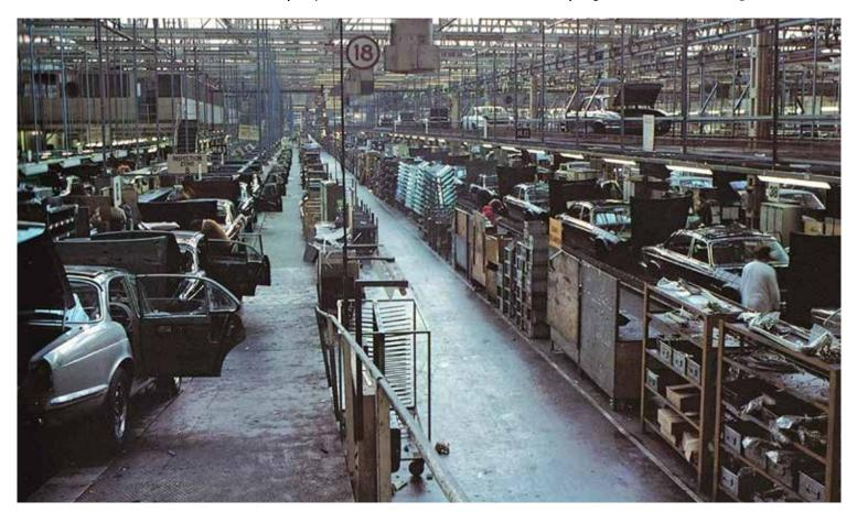
XJ production line. The bodies were lowered onto the engine and front and rear suspension - much the same as was originally introduced in the assembly of the Mark 1. With all mechanical components in place, the final production line saw the remaining items of trim and minor accessories installed. Then came road testing and final inspection.
