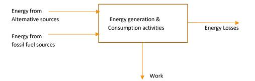
Under the general energy balance equation, the sum of the energy inputs equals the sum of the energy outputs. So, when considering the general energy balance for such a simple system, one can see how energy inputs can be reduced by: increasing the energy efficiency of the facility (i.e., reducing energy losses), reducing the energy requirements of the unit operations of the facility (i.e., reducing the amount of "work"), or increasing energy usage from alternative sources.
