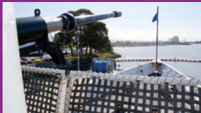
(Above) Among Morganthau's weaponry is this 76mm deck gun that can fire 80 rounds per minute out to 10 miles.
