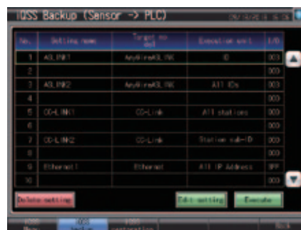
iQSS backup (sensor -> programmable controller) screen
