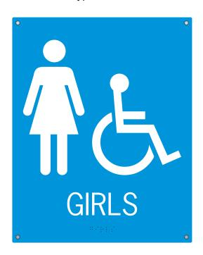
.060" stainless steel, 1/16" radius corners die-cut w/ burr side down. Embossed text raised min. 1/32", embossed domed California grade 2 braille min. 1/40". Epoxy powder coated blue background w/ white copy.
