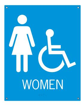
.060" stainless steel, 1/16" radius corners die-cut w/ burr side down. Embossed text raised min. 1/32", embossed domed California grade 2 braille min. 1/40". Epoxy powder coated blue background w/ white copy.
