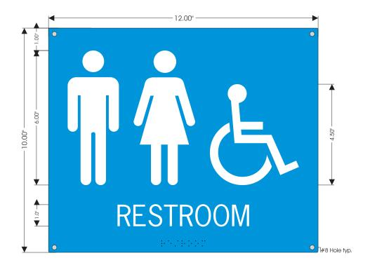
.060" stainless steel, 1/16" radius corners die-cut w/ burr side down. Embossed text raised min. 1/32", embossed domed California grade 2 braille min. 1/40". Epoxy powder coated blue background w/ white copy.
