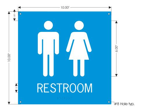
.060" stainless steel, 1/16" radius corners die-cut w/ burr side down. Embossed text raised min. 1/32", embossed domed California grade 2 braille min. 1/40". Epoxy powder coated blue background w/ white copy.
