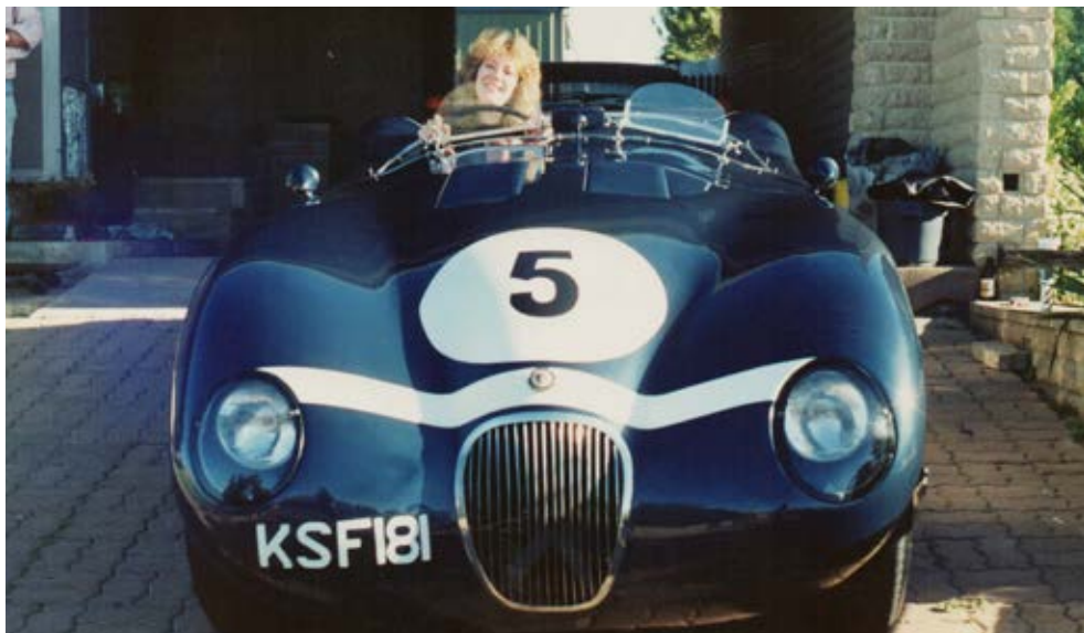
Val Weeks in the ex Gavin-Sandford-Morgan, ex John Blanden Ecurie Ecosse C-Type Jaguar. The XK120-C's were designed by Malcolm Sayer, but Lyons required the addition of a grille similar to the XK120 to align the C-Type with the road going car (and assist sales).
