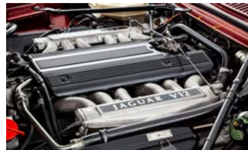
1971 (5.3L) & 1994 (6.0L) V12 engine. Overtime the engine and accessories were "tidied up" and made significantly neater.
