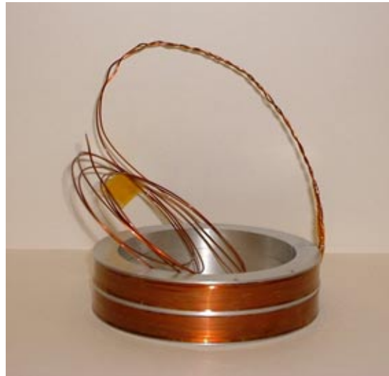
Figure 7.6: Field winding with aluminum bobbin.
