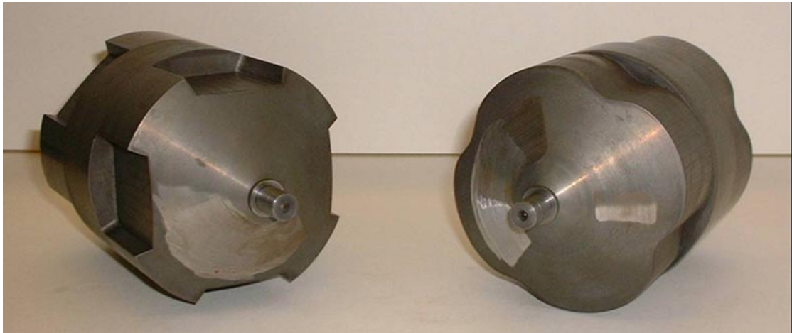
Figure 7.2: Photo of squarecut and sinusoidal rotors. Although they have different pole profiles and MMF waveforms, both rotors have 8-poles and have no saliency ( L_d/L_q=1 ).
