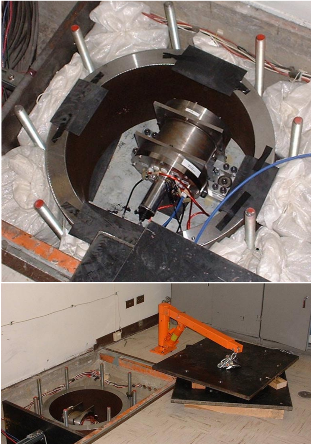
Figure 7.13: Photo of motor inside the containment pit (top) and photo of containment pit lift and top plates (bottom). When conducting high-speed tests, the top plates (bottom photo, right) are put into place using the hydraulic lift (bottom photo, top).
