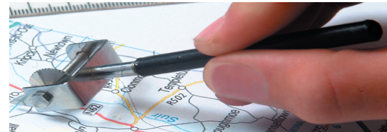
Opisometer - measures curved lines
