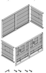
NOTE: For Steps 1 and 2, the **cage body** will be assembled UPSIDE DOWN for ease of assembly.
