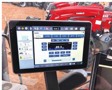
The Magnum's Surveyor cab has 360 viewing and a new level of digital connectivity by way of the 12-inch AFS Pro 1200 display.
