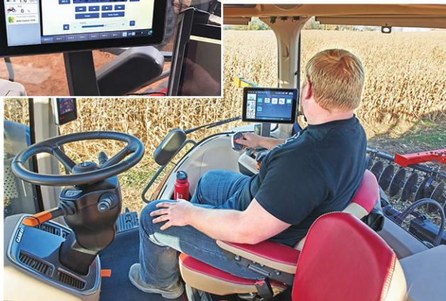
The Magnum's Surveyor cab has 360 viewing and a new level of digital connectivity by way of the 12-inch AFS Pro 1200 display.
