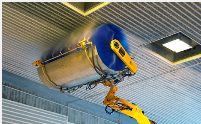
The tunnel washing brush TWB 2100 also cleans tunnel ceilings effectively.
