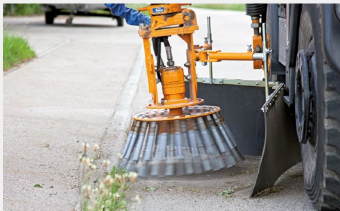
The weed brush WKB 750 is clearing outgrowth at road kerbs.
