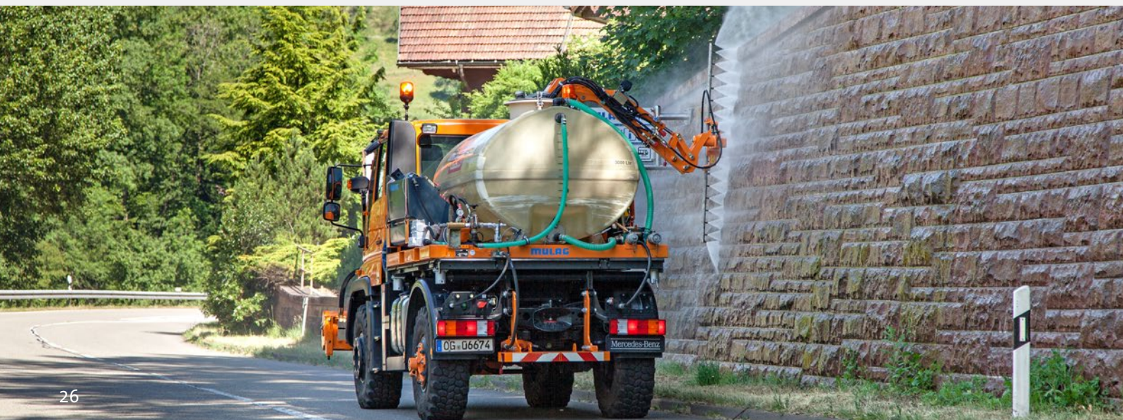
Three-section high-pressure spray bar in use on a tunnel wall
