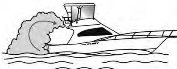
Figure 3. When protective weather coverings are in place, engine or generator exhaust from your yacht, while docked and/or running, can cause excessive accumulation of Carbon Monoxide gas within the cabin and cockpit areas of your yacht. Always provide adequate ventilation when the weather coverings are in place and either the engine or generator are running.
