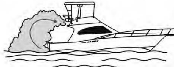
Figure 5. Engine or generator exhaust from your yacht while underway at a slow speed can cause excessive accumulation of Carbon Monoxide gas within the cabin and cockpit areas of your yacht. A tail wind can increase the accumulation. This is often referred to as the "station wagon effect". Always provide adequate ventilation or increase your speed if possible.
