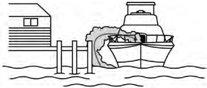
Figure 1. Blocked hull exhaust outlets near a pier, dock, seawall, bulkhead or any other structure can cause excessive accumulation of Carbon Monoxide gas with the cabin areas of your yacht. Be certain hull exhaust outlets are not blocked in any way.
