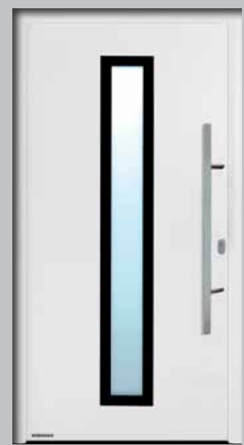
Style 600 ■ NEW from 1.7.2017 Stainless steel handle HB 38-2 on steel infill, with surface-mounted glazing: triple-pane insulated glass, exterior laminated safety glass, centre sand-blasted float, interior clear single-pane safety glass, U_D -value up to 1.1 \text{ W}/(\text{m}^2\cdot\text{K})^*
