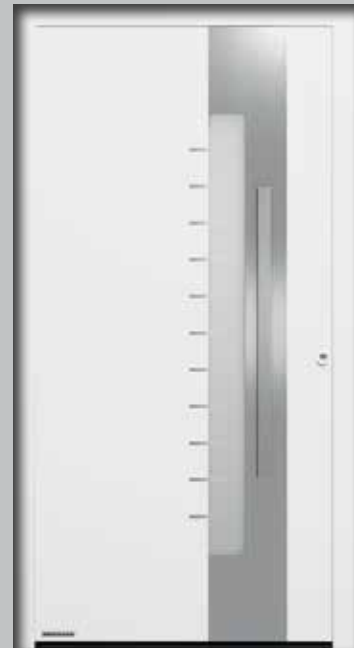
Style 560 Stainless steel handle HOE 600, stainless steel embellishment, matt design glass with 11 clear stripes, triple thermal insulation glass, U_D -value up to approx. 0.9 \text{ W}/(\text{m}^2\cdot\text{K})^*
