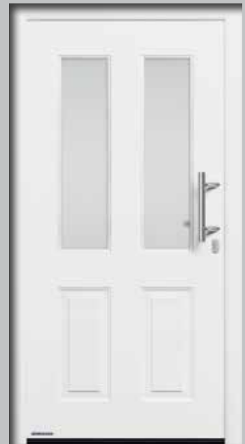
Style 410 Stainless steel handle HB 14-2 on steel infill, triple-pane insulated glass, exterior laminated safety glass, centre sand-blasted float, interior clear laminated safety glass, U_D -value up to approx. 1.0 \text{ W}/(\text{m}^2\cdot\text{K})^*
