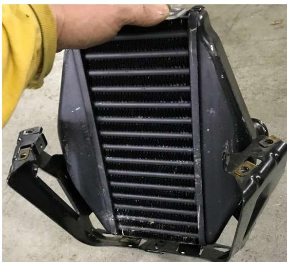
4. Attach the isolators to the front mounting plate of radiator assembly. Isolator stud goes through the slotted hole on mounting plate. Do not tighten the nuts real tight as the isolators need to be free to float initially.
