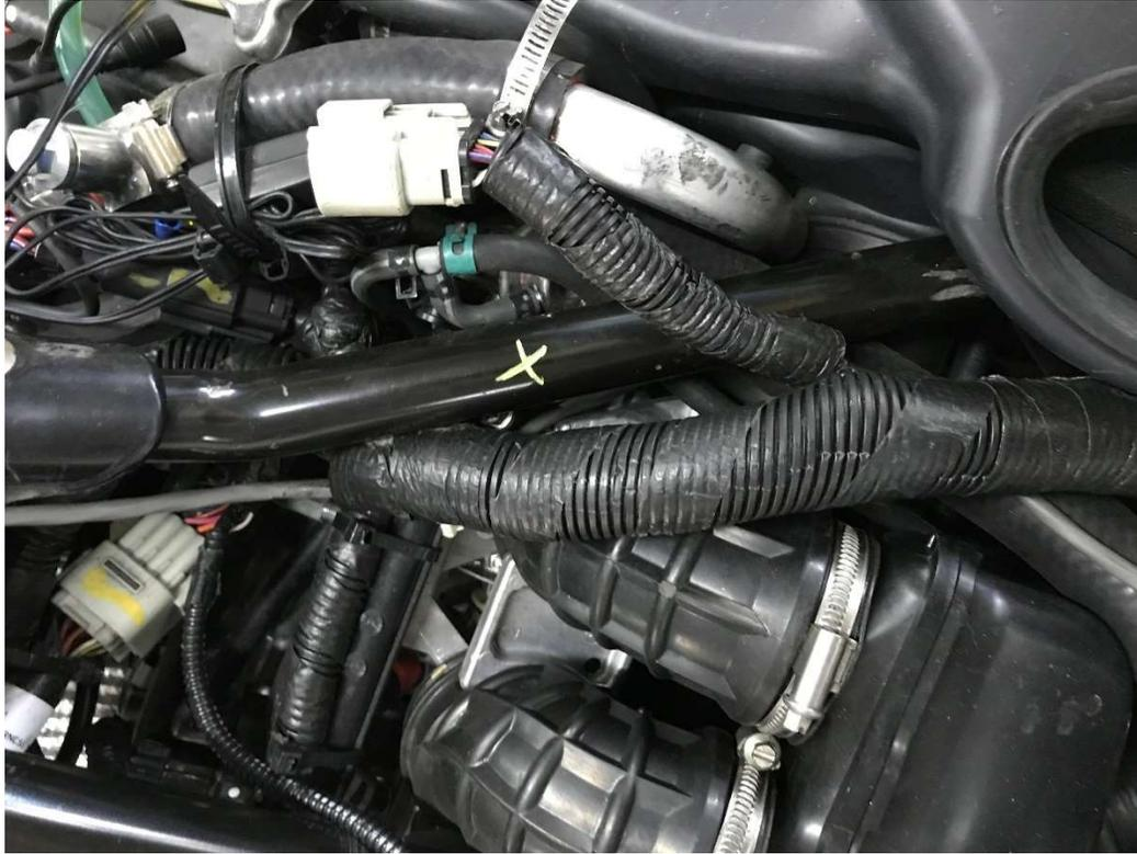
9. Next mount the fuse box next to the radiator as shown below. You can rivet the bracket to the black plastic.
