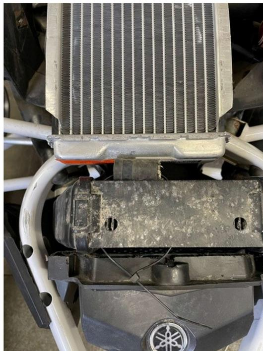
16. Once intercooler is installed set the hood next to sled and plug it back in so the sled can be run. Start the sled and let it get up to temperature. Check to ensure all hoses get hot and coolant is circulating. Coolant will flow as follows: thermostat housing to clutch side of radiator to clutch side of tunnel cooler to throttle side of tunnel cooler to front tunnel cooler. Check all connections for leaks.
