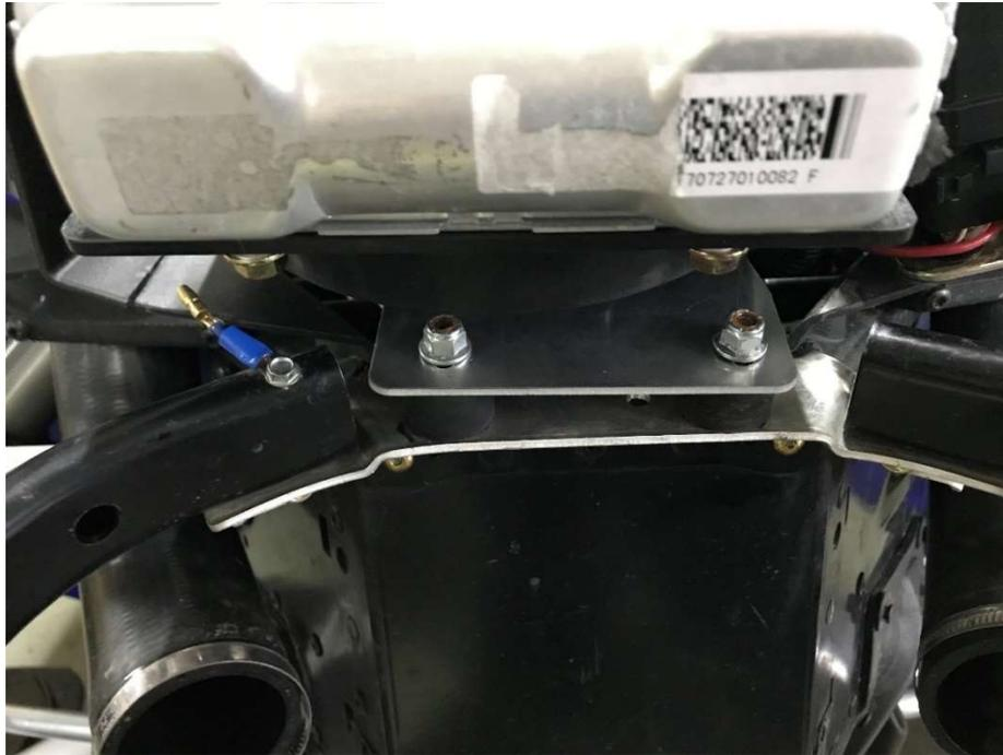
6. Remove the radiator assembly. Align the isolator template with the markings made in step 6. Once template is in place tape it on and center punch the center of each isolator. Remove the template and drill a  $\frac{1}{4}$ " hole through each center punch mark.
