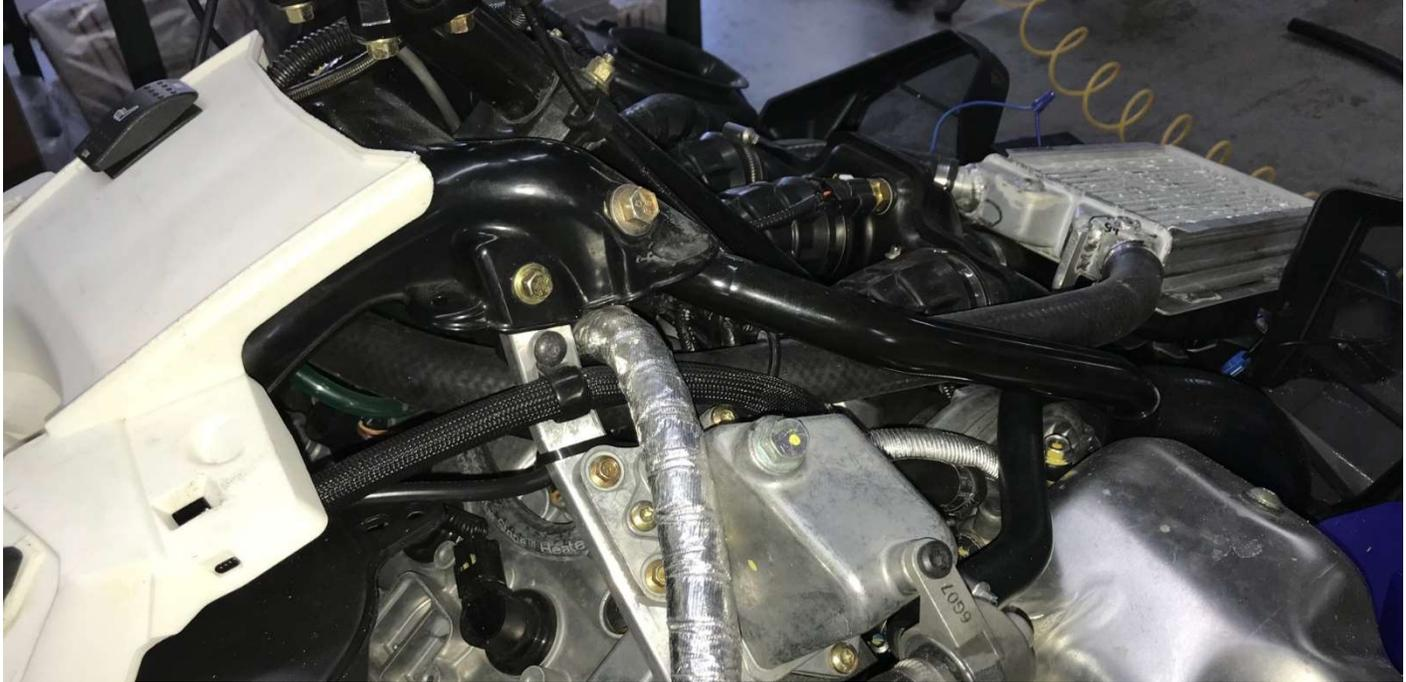
13. Ensure all clamps are tight and then proceed to add coolant. Start by filling the system with the oem fill cap. Add coolant until it is topped off. Once the oem fill point is topped off, the T fitting becomes your new fill point. The t fitting is the highest point in the radiator loop and will self bleed. Remove the bolt on the top of the fitting and using a small funnel fill the system. Pouring slowly helps allow air to bleed out.
