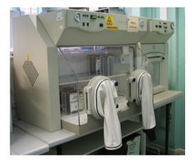
Figure 23.7 Anaerobic cabinet used for growing anaerobic bacteria.
