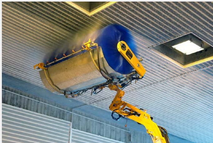
The tunnel washing brush TWB 2100 also cleans tunnel ceilings effectively.
