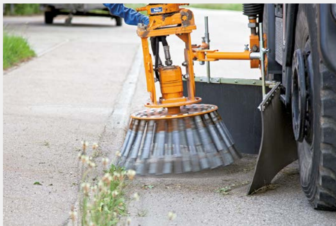
The weed brush WKB 750 is clearing outgrowth at road kerbs.
