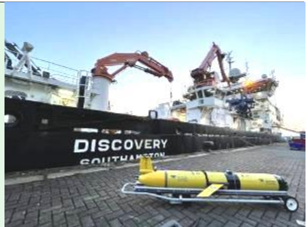
Underwater gliders, deployed from RRS Discovery, have contributed to global research on the ocean carbon cycle. (Photo credit Filipa Carvalho as part of the GOCART Project)
