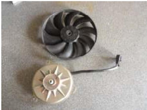
4. Next attach the fan motor to the shroud using the (3) M5 bolts and lock nuts. Orient the motor so the wire lead is at approximately 11 o'clock position. Then install the fan blade back onto motor.
