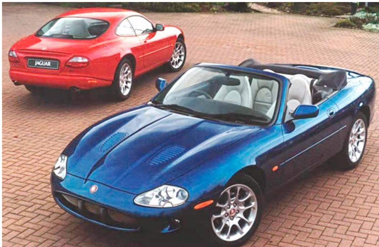
In 1998, two years after the XK8, came the XKR which featured an Eaton supercharger, mesh grille, larger wheels and bonnet louvres.
