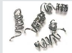
Loosely coiled chips are a sign of ideal cutting conditions.
