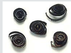
Thick, heavy or bluish chips signal overstressing of the saw blade.
