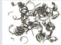
Very fine or pulverized chips indicate that cutting pressure is too low.
