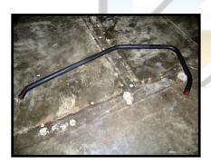
The roll bars consist of several pieces. There are two large pieces (left). Start with one of these and then the other before assembling the other roll bar components. Use
