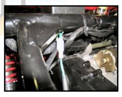
connection is located, plug them together. Run the brake light wire into the wire holders underneath the rack's center for aesthetic value.
