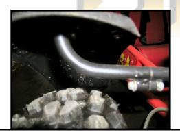
The front fenders go behind the front tires. On the right, the fender connection point is in the
