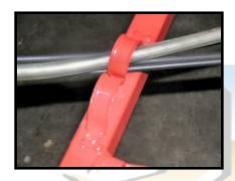
Before installing the seats, remove this unused wire brace because it gets in the way otherwise.
