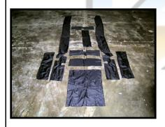
Using this picture, the location of any piece can be identified. Install these vinyl covers onto the roll bars.
