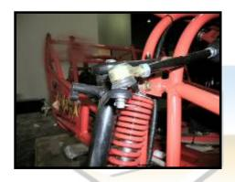
Place the bolt into the hole and tighten the nut. Insert a cotter pin into the hole at the bottom of the steering rod attachment bolt. Repeat for the other side.
