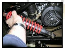
The bottom of the shock should already be attached to the frame.
