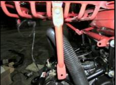
Remove the bolts from the connecting arms of the rack.
