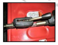
Remove the parking brake assembly from the bracket and place it to the side.
