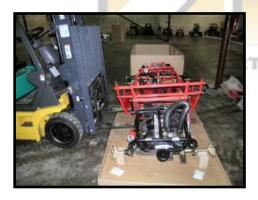
Raise the rear of the frame using a forklift or a jack until the engine compartment swings down a bit. Do not lift the black engine compartment frame portion because the pivot point is where it connects to the kart's main frame.
