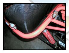
The other end of the longest roll bar component connects just above the rear shock behind the seat (the connection point described above is located in the top right in the picture on the left).
