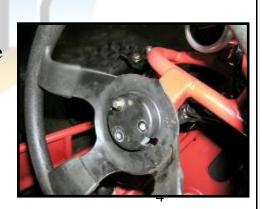
The steering wheel spokes should extrude toward the driver with the middle spoke pointing down. Bolt it into place. Install the aesthetic cup found in the small box earlier.
