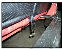
The center seat belt connector should come through the space between the seats. The center seat belt connection bracket is underneath the seats on the frame's center cross member.
