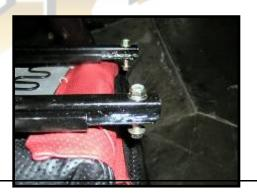
the rear of the seat as possible while still being able to lock down the seat adjustment mechanism. Remove the nuts and bolts from the sliding braces underneath the seat.
