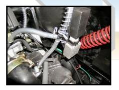
The other rubber hose coming from the gas tank connects to a T shaped connection.
