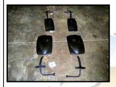
On the left is a picture of the fender components. Assemble these using the nuts and bolts in the small box. The bigger sized ones go on the front side of the back tires. The back fender connects here (right/below).
