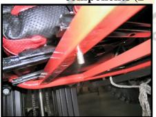
The first bolt should be placed on the same side as the seat adjustment handle (top left) into the sliding brace and frame anchor point (left). Thread the nut on loosely to facilitate adjustments while doing the other side. Tighten them both
