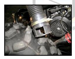
Locate the snorkel and loosen the bracket. Remove the top of the snorkel. Locate the loop that secures the snorkel on the rack. Run the snorkel through, replace the top, and tighten the bracket.
