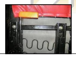
The seat adjustment lever is underneath the seat near the front. Use this to extend the sliding braces as far towards
