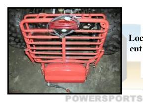
Locate the rack and carefully cut the plastic packaging ties off.
