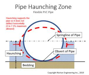
FIGURE 3: PIPE HAUNCHING ZONE FOR FLEXIBLE PIPE
