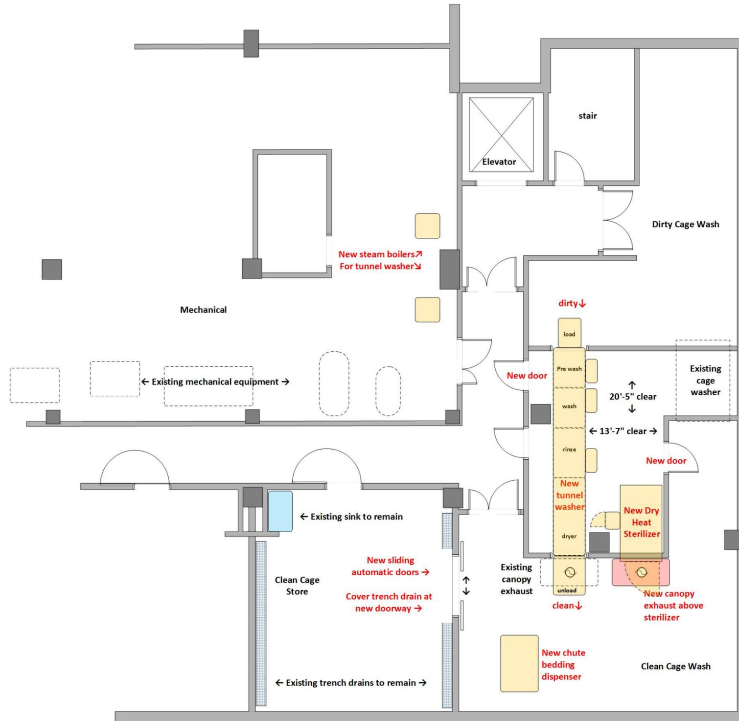
Similar to scheme A, but reverses location of dry sterilizer and tunnel washer. This scheme requires a new door at northwest corner of tunnel washer room.
