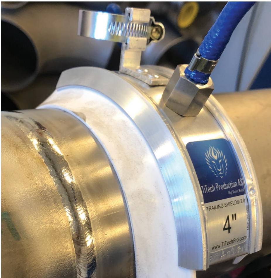
☑ Titanium Grade 2 welded by Glenn Hovet with second generation Trailing Shield 2.0™ from TiTech PRO™.
