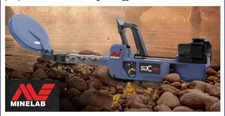
The SDC 2300 is very sensitive to small gold scattered in heavily mineralised ground. This gold is often missed by prospectors with both VLF and PI detectors because of the difficult ground conditions and fine gold size.
