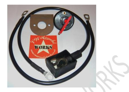
The battery isolator switch comes with the battery isolator, stainless steel mounting plate, 2 x 0.5 metres battery cable and fastenings. One cable has 10mm rings on both ends and is for connecting to the vehicle body, the other cable has a 10mm ring for connecting to the isolator and the other end connects onto the negative terminal of the battery.
