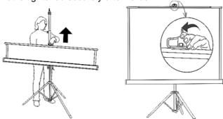
6. Hang the handle on the suspension hook in one of the notches. The angle of the screen can be adjusted by placing the handle in different notches.
