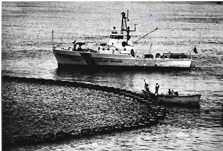
The venerable 82-footers were used for nearly all Coast Guard missions for more than 30 years. Here an 82-footer is used as a platform for the testing of a floating barrier designed to keep oil pollution from spreading.
