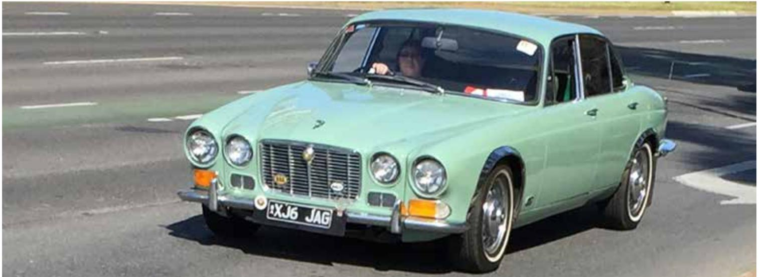
*1971 Series 1 XJ6 featuring the deeper grille, slender bumpers and chrome overriders. Production changes in 1970 included modifications to the front wheel arch flanges to provide better tyre clearance.*
