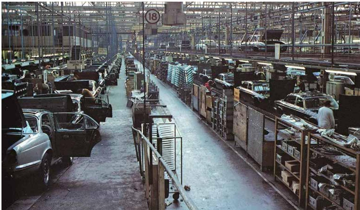
*XJ production line. The bodies were lowered onto the engine and front and rear suspension - much the same as was originally introduced in the assembly of the Mark 1. With all mechanical components in place, the final production line saw the remaining items of trim and minor accessories installed. Then came road testing and final inspection.*
