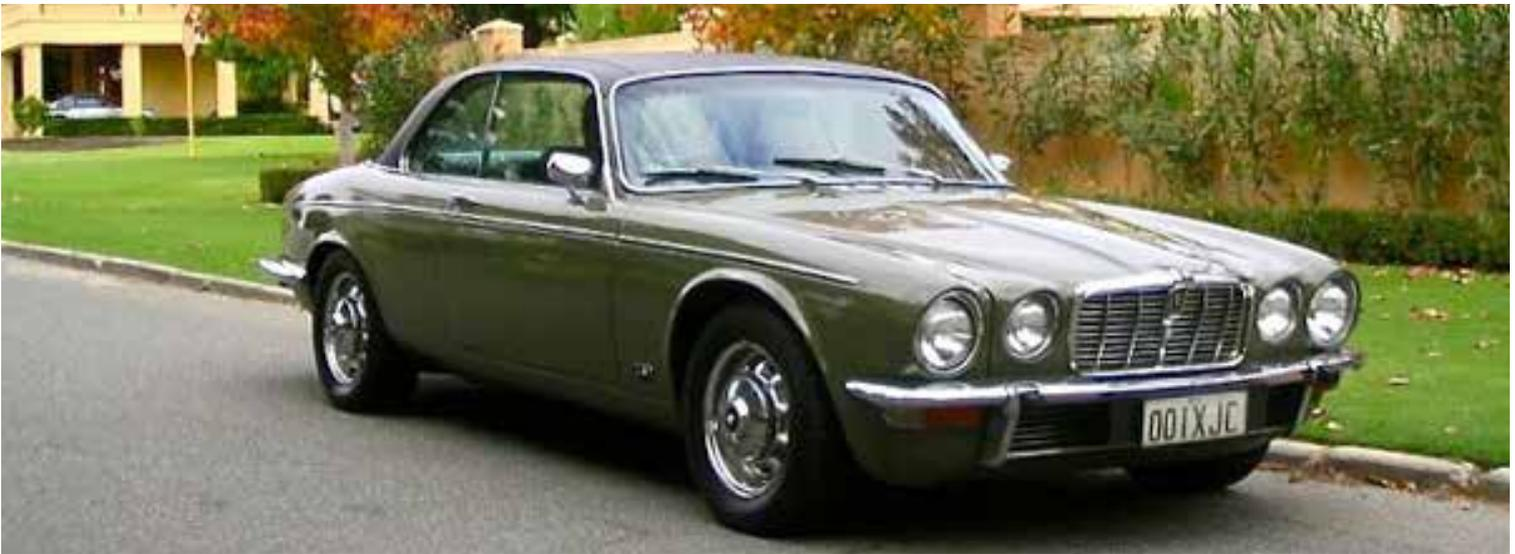
*1978 Series 2 XJC. To comply with US safety regulations, a higher front bumper and smaller grille was fitted. The overriders became 'underriders' flanking a prominent rectangular air intake with indicator lights under the bumper.*
