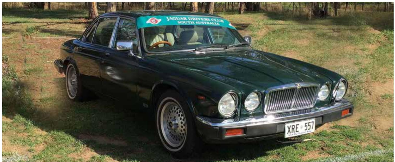
*1985 Series 3 XJ6. The most obvious changes were the injection-moulded black bumpers with integrated indicator lights, flush door handles for increased safety and a revised roofline with narrower door frames and increased glass area.*
