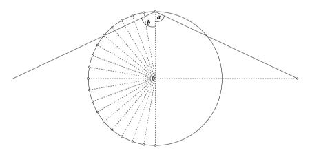
4. Repeat step 3 for the other circumference points, measuring angles from the other pencilled radius lines. Finally, erase each radius. The remaining lines should 'stitch' a caustic curve.
