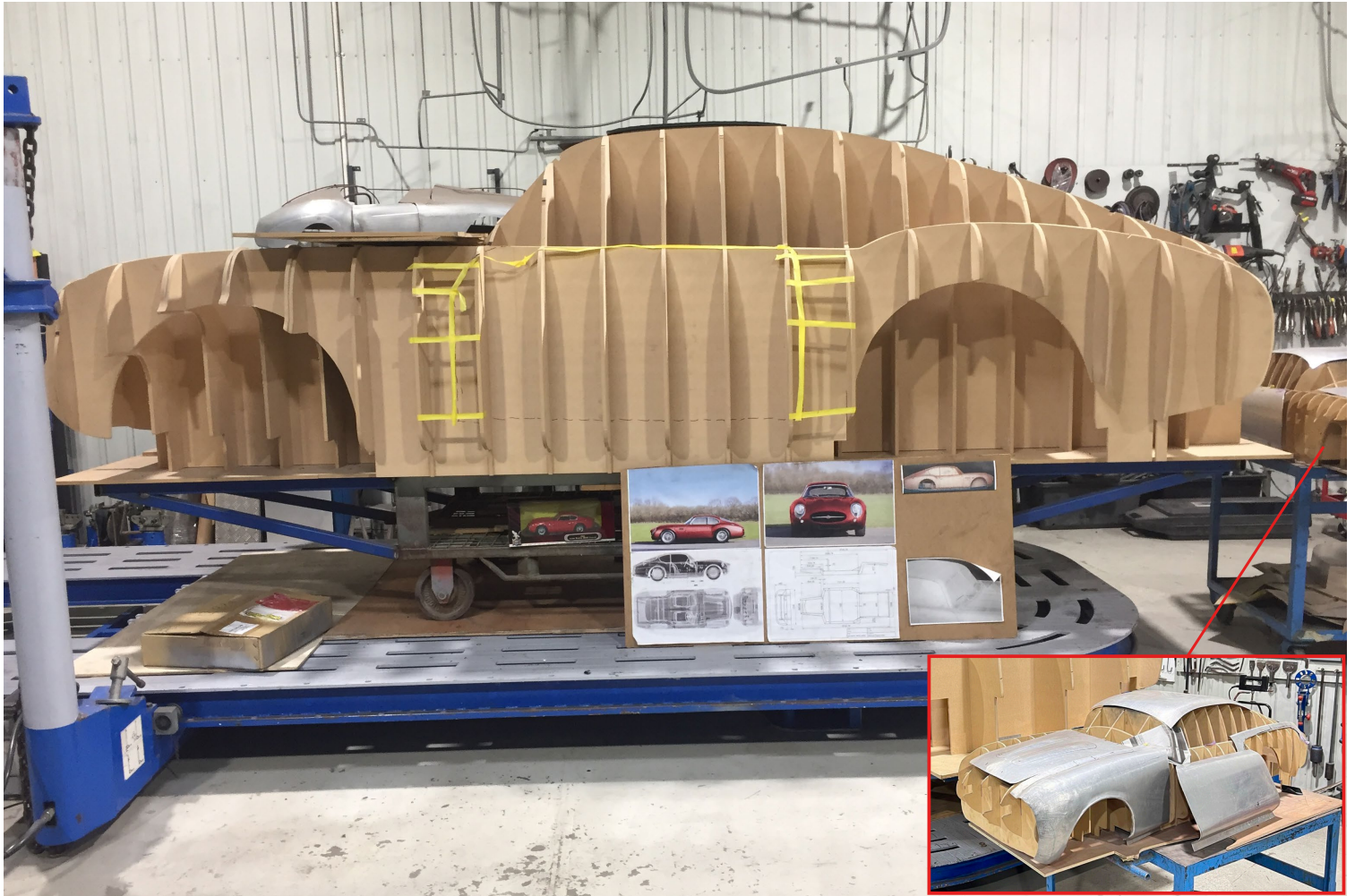
Marque Restorations will be fabricating a complete car built on a section of Jaguar Mark IX chassis with the design as shown in the photos. Two timber bucks have been made, a miniature to see what the final car will look like and the other being full size for the final fabrication.
