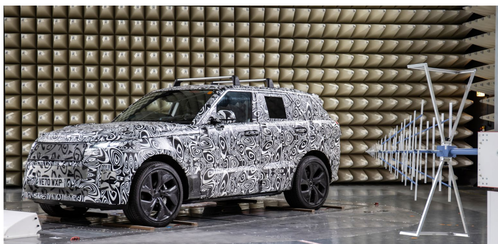
New JLR drive-in EMC RF anechoic test chamber.
