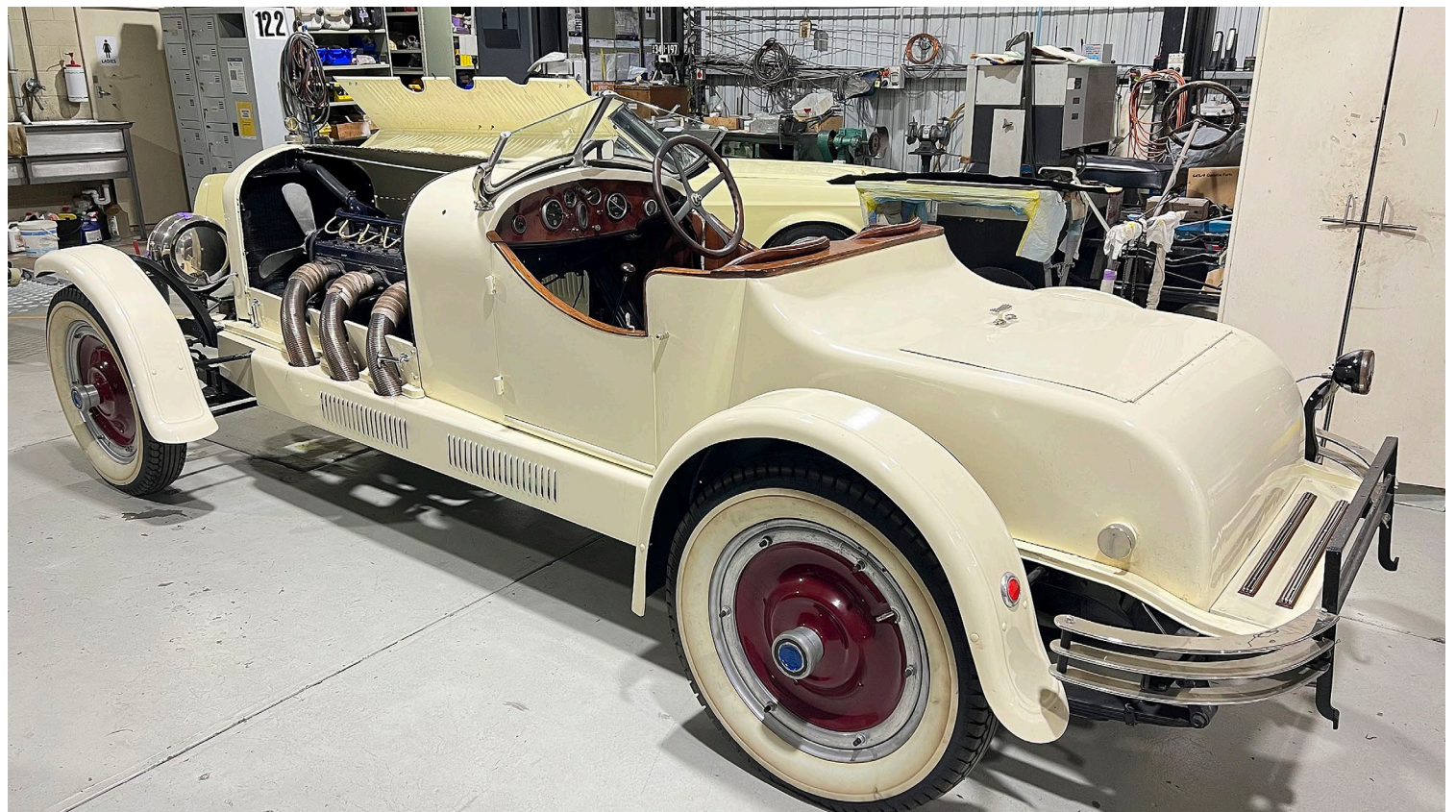
A particularly rare Flint - an automobile marque that was assembled by the Flint Motors Division, Flint, Michigan between 1923 and 1927. This particular model is powered by a 6 cylinder Continental side valve motor.
