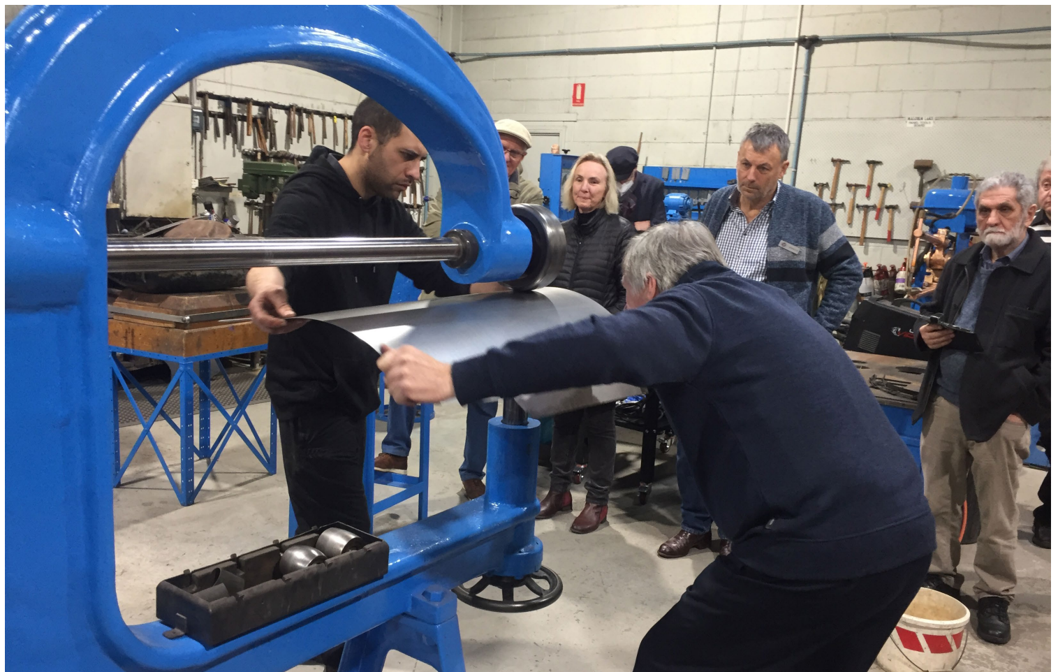
Gerard and "T" kindly provided a demonstration on how to fabricate an E-Type door skin from a sheet of aluminium. Amazing!
