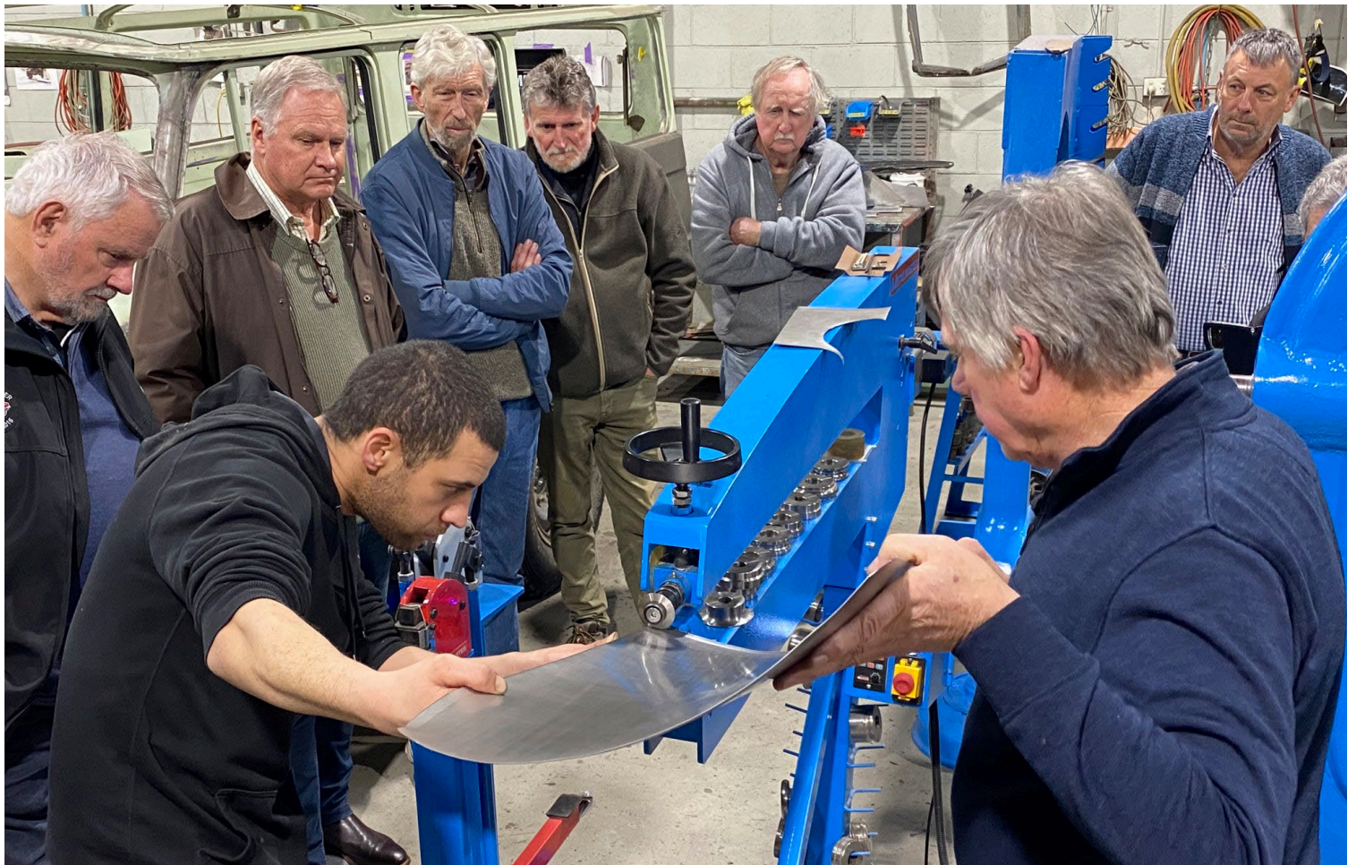
Gerard and "T" kindly provided a demonstration on how to fabricate an E-Type door skin from a sheet of aluminium. Amazing!
