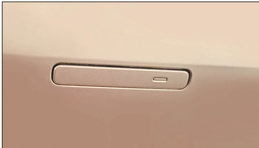
Flush-fitting door openers for the I-Pace are activated with a light press
