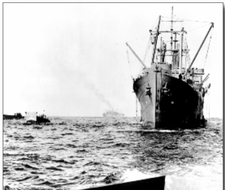
Rare photograph of the USS Hunter Liggett debarking troops for the Guadalcanal landings. Notice the use of cargo derricks to lower landing craft into the water. (Courtesy of the U.S. Navy)
