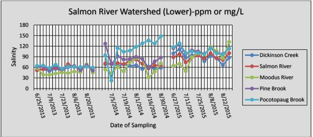
**Quick Summary:** In general, salinity shows an upward trend for most stream segments. This may be partially explained because compared to 2013, 2014 had less precipitation and 2015 had less than 2014. Since salinity is related to conductivity, please see the Quick Summary on that section to read about a further step we are taking to address this upward trend.
