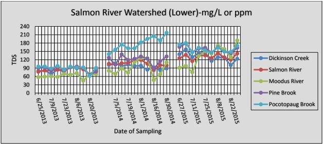
**Quick Summary:** In general, total dissolved solids show an upward trend for most stream segments. This may be partially explained because compared to 2013, 2014 had less precipitation and 2015 had less than 2014. Since total dissolved solids are related to conductivity, please see the *Quick Summary* on that section to read about a further step we are taking to address this upward trend.
