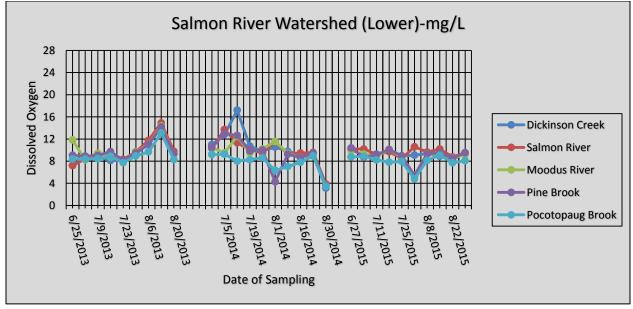
**Quick Summary:** Gaps in data indicate instrument malfunction. In general, DO ranges showed more variability in the summer of 2014 versus the summer of 2013, but less in the summer of 2015. In 2015, readings dipped the lowest in the season around 7/31 and 8/1, corresponding with the highest water temperatures. Ranges in the 3-5mg/L can be stressful for fish populations.
