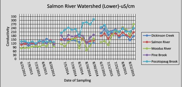
**Quick Summary:** Gaps in data indicate instrument malfunction. In general, conductivity shows an upward trend for most stream segments. This may be partially explained because compared to 2013, 2014 had less precipitation and 2015 had less than 2014.
