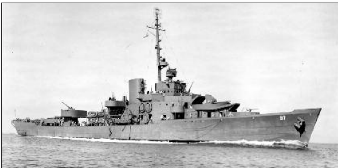
USCGC Taney underway at the time of the Baker Island survey, July 1943. At this time of the war, her main armament consisted of two 5"/51 caliber guns, four 3"/50 caliber dual-purpose guns, seven 20mm AA guns, plus depth charge throwers and tracks.
